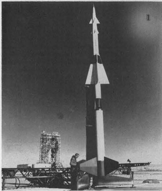
In operation the Nike battery (Fig. 1) is alerted by the air warning net that hostile planes are approaching the area. The target is picked up and tracked electronically. Meanwhile the Nike's missiles are readied in vertical position and a running account of the target's changing
